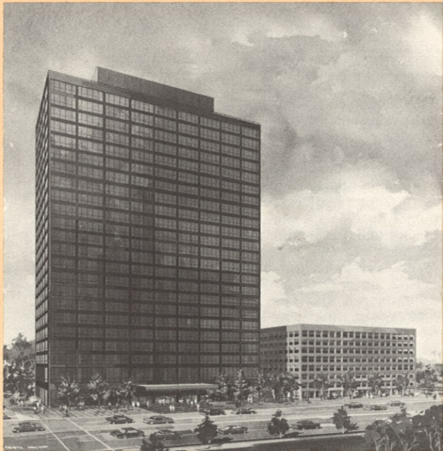
Tishman Westwood, Los Angeles, California. 13 Montgomery gearless passenger elevators with speeds up to 800 fpm serving 24 floors.
